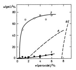
Fig. 1. A plot of the gel content in crosslinked isotactic polypropylene vs. BP (1) and DCP (2) mass fraction at constant w(PETA) = 4 %. A — dependence of the gel content on dibenzoyl peroxide mass fraction; B — dependence of the gel content on dibenzoyl peroxide mass
