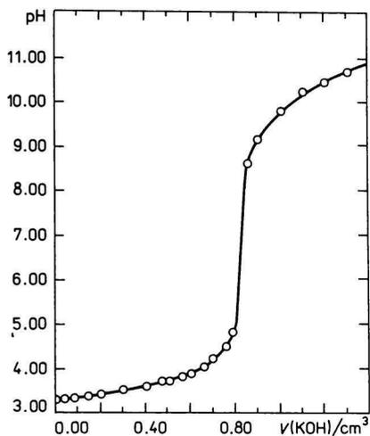
Fig. 1. Course of titration curve for titration of  $\text{H}_2\text{EBDTC}$  acid with KOH solution.
