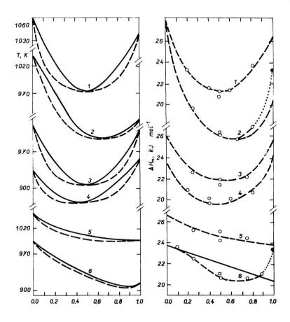
*Fig.* 1. Phase diagrams and heats of melting of the solid solutions. 1 NaCl—KCl; 2. KCl—CsCl; 3. NaBr—KBr; 4. Nal—KI; 5. KCl—RbCl; 6. RbCl—CsCl.  $\Box$  Calculated values;  $\bigcirc$  experimental values;  $\bullet \Delta H_m$ (CsCl)— $\Delta H_{trans}$ (CsCl).
