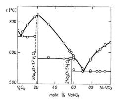
Fig. 1. The phase diagram of the system  $V_2O_5-NaVO_3$ .
