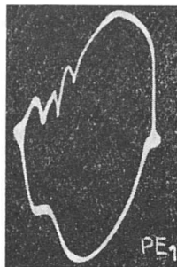
Fig. 1. dE/dt = f(E) curve of 10^{-3} M melamine solution in 1 M-KCl.
